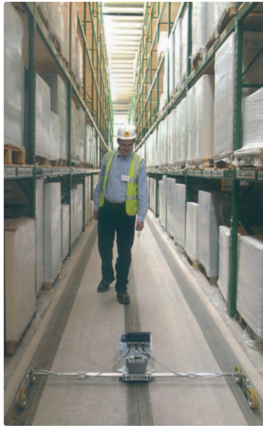
Figure 3 right: Face TR 34 digital profileograph checking compliance with Table 4.3. Only the outer two wheel tracks are tested.
