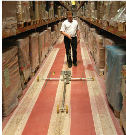
EXACTING TESTS TO DETERMINE FLOOR FLATNESS.
